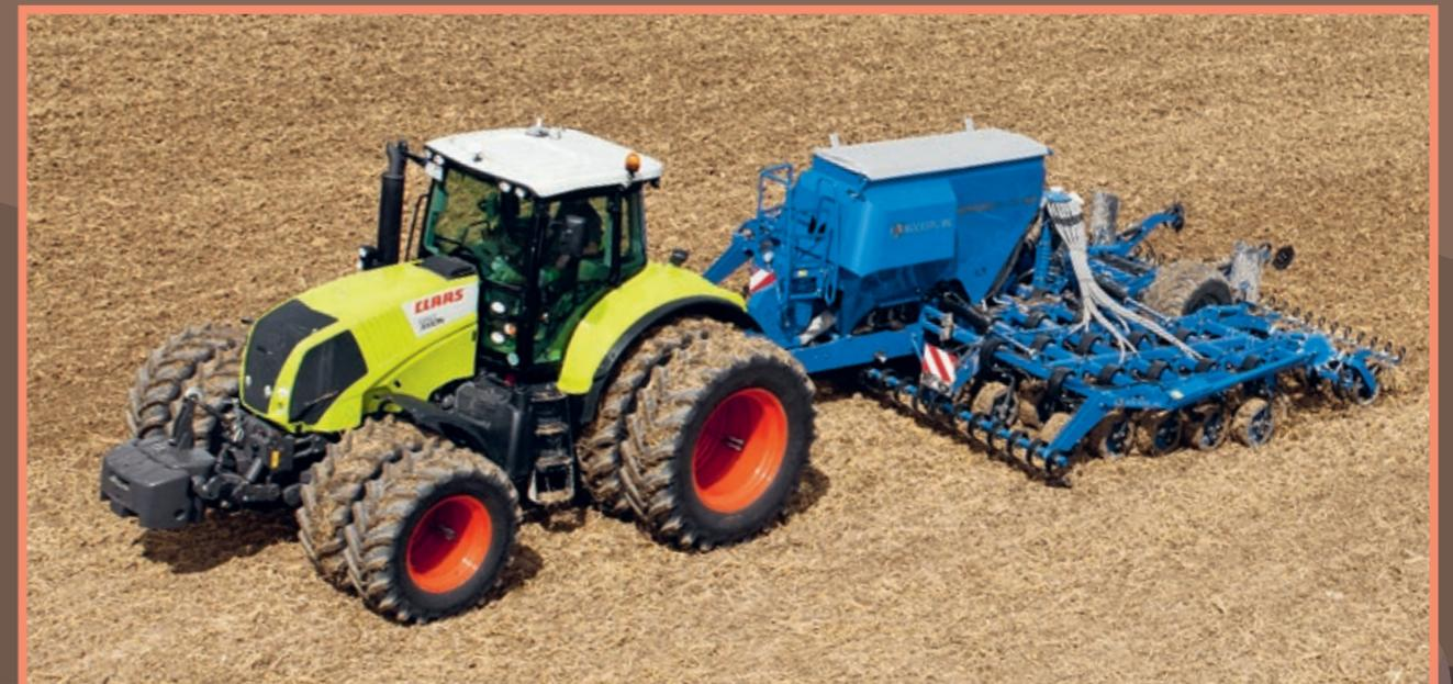
DER SCHLEPPER IST MIT ZWILLINGSREIFEN UNTERWEGS. DAHINTER HÄNGT EINE DRILLMASCHINE, DIE RINNEN IN DEN ACKER ZIEHT UND DARIN SAMENKÖRNER ABLEGT.
